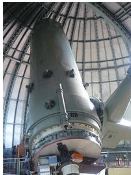
The 1.93m(76") reflector telescope, the largest at the Haute-Provence Observatory Information and image from Wikipedia
