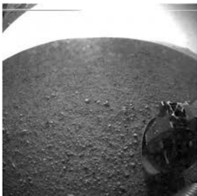
Left-one of the first images taken from the surface, only a few minutes after the rover landed. It was taken by the black and white low resolution landing camera to ensure that the craft was safely on the surface.
